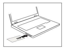
Slide the SmartCard into the SmartCard reader with the chip facing upwards (on some variants it faces down) and to the front.
